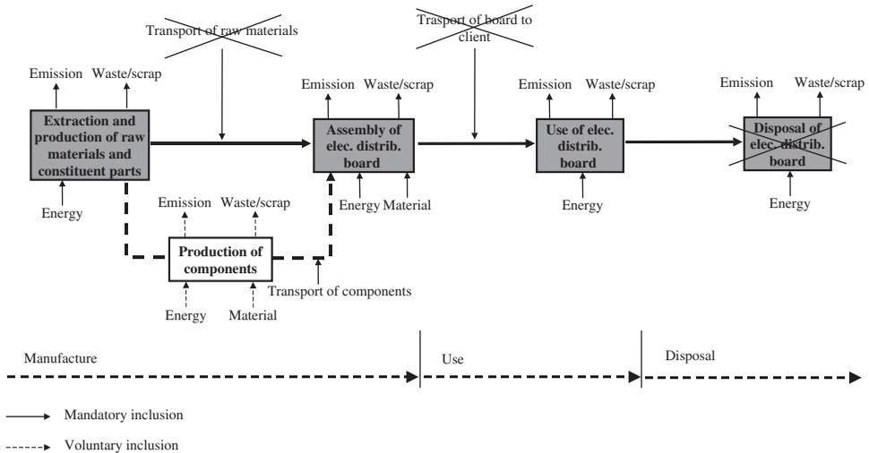
Figure 3. Electrical distribution board life cycle flow chart.
