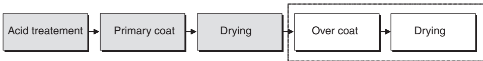
Figure 5. Two omitted processes in painting process flow when high solid paint is applied in the painting process.
